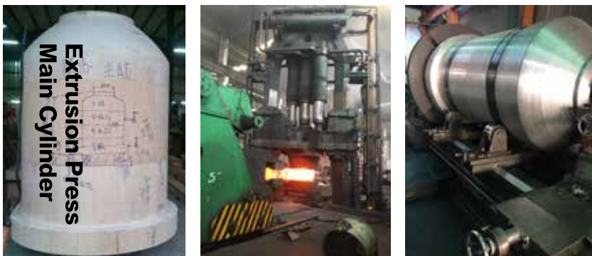
Figure 9: Wooden mold, casting steel bar for forging, and NC processing.
